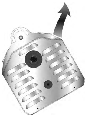
Figure 2.9 • Hot Flue Discharge
