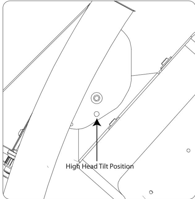
To set heater head angle at high position, manually push heater head up to align hole then insert slip pin.
