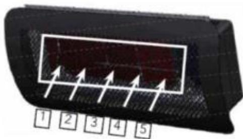
3. Clean burners: Burners can be cleaned by directing compressed air (max20PSI) at outlet ports. Avoid directing air at gasket material between ceramic tile and burner cup.
