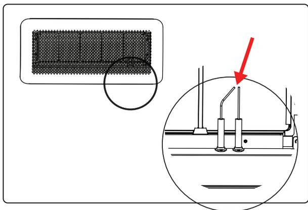
5. Once at IGNITION position, press control knob while simultaneously pressing the spark ignition button. Continue to hold in controls for 10 seconds for ignition to complete.
