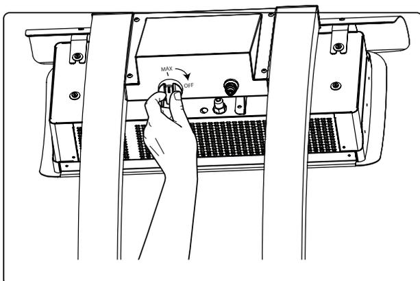
2. Turn OFF the gas supply at the LPG storage bottle or disconnect natural gas supply hose from natural gas supply
