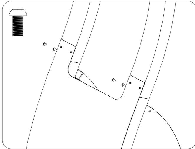
\* Note: The joint between the lower and upper arms is firm to ensure rigidity and stability of the product. To engage slowly lever the two sections together using some force and push down fully
